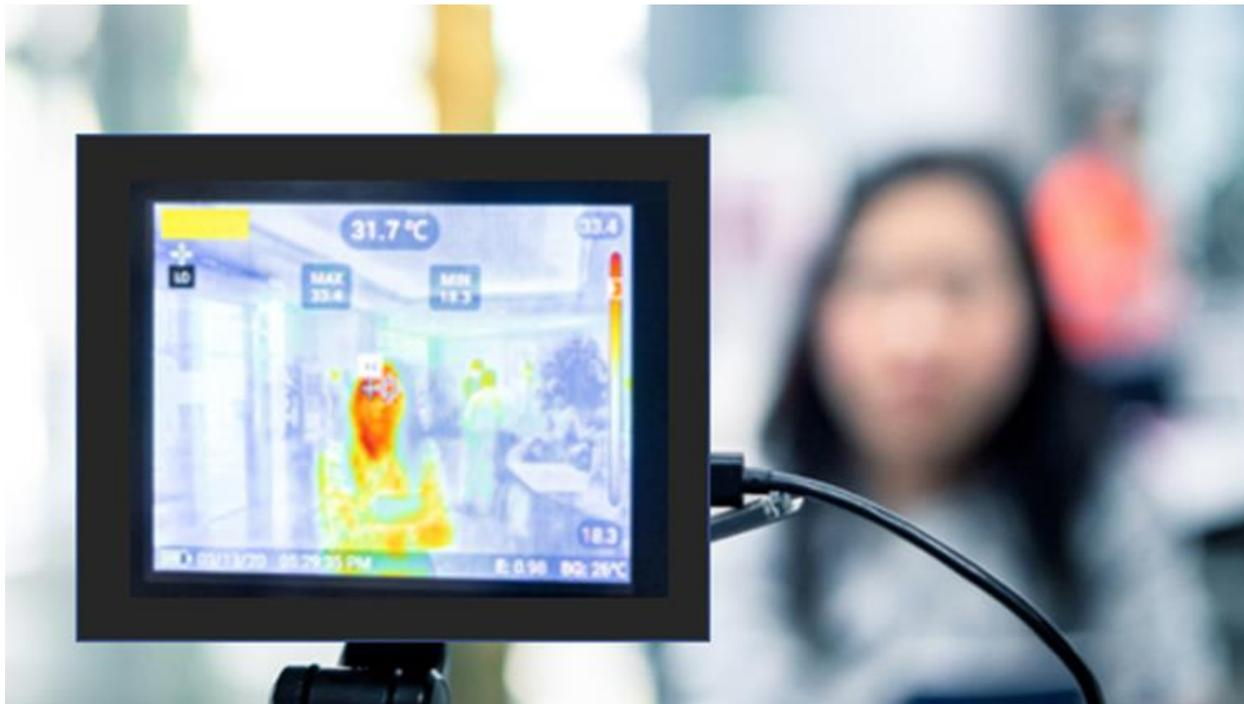
Thermal imaging systems can either be handheld or fixed. Fixed or “standoff” systems screen the subject at a distance, making it safer for the operator. Fixed systems consist of an imaging camera, a processor, and software. The software can be used to increase the accuracy of the scan by comparing the temperature to a known database of normal temperatures for the area.
